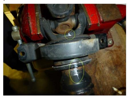
**Step 4**. Now it's time to get out the hammer. Hit the end of the driveshaft away from the bearing (see below image) until the two halves have separated. I'm not going to lie, this will be the most difficult thing to do during this repair. It's going to take time and some elbow grease to get done. As it separates it will begin to look like the second image.
