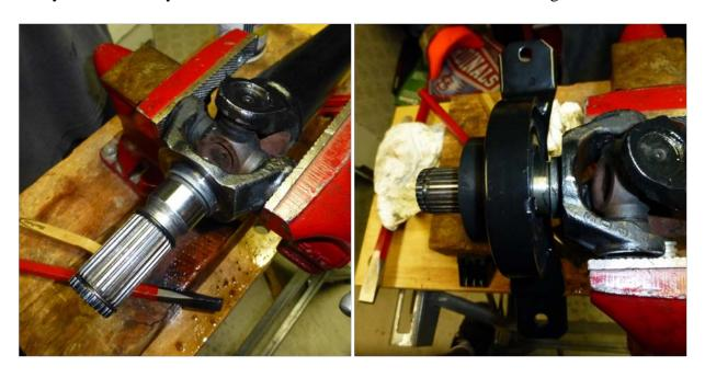
Next, realign the loose end of the drive shaft with marks that you made earlier and slide it up as far as you can. With a block of wood at the other end, hammer the driveshaft and bearing back into place.
